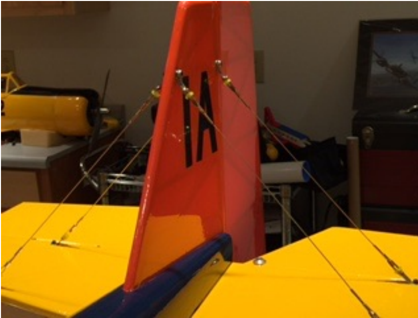
Getting better at soldering. Tail also has wires on the bottom side. Makes for solid section.
